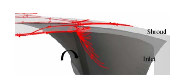
图 25 c=0 mm,前排叶片叶背分离流动(设计点) Fig. 25 c=0 mm, the flow of separation at FB (design point)
